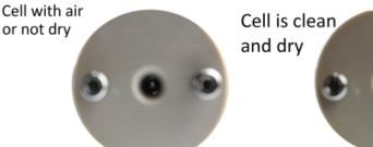
Of course my description assumes that we are going to clean the polarimeter cell immediately after measurement however people are people and mistakes happen. Sometimes samples precipitate in the cell, sometimes people forget to clean the cell and the sample dries on the cell wall. This section shows how to pull the cell apart if simple cleaning does not suffice
